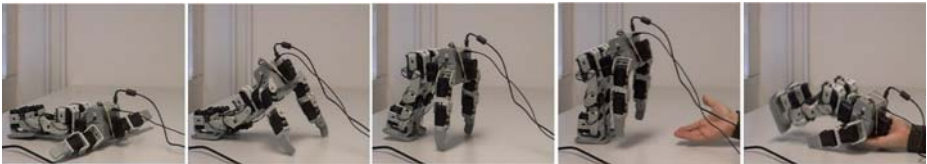
Fig. 3. Direct replay of a demonstrated standing up skill by the small humanoid robot. The robot fails to stand up, because of the missing support forces of the human teacher.
