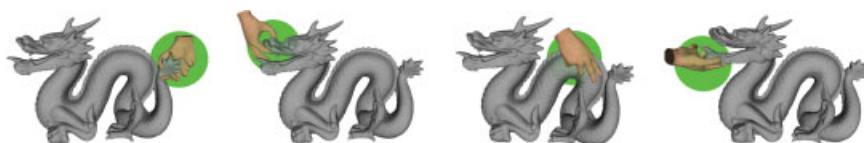
Figure 6. The results of applying grasp optimization on the Stanford dragon model. The position of the hand and the area of interest (green) were specified by the user. Both the hand shape, and orientation were computed by the optimization process.
