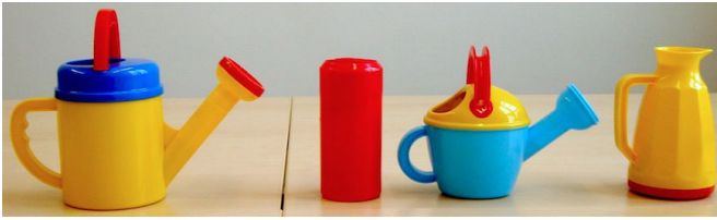
Figure 2. The picture shows the four objects used in the pouring task experiment. The robot was initially shown how to pour with the large watering can on the left. The robot then had to autonomously learn to generalize this demonstrated action to the three objects on the right: a plastic cup, a different watering can, and a small jug.
