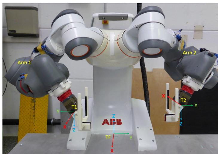
**Figure 12.1:** Locations of the task frame **TF** and the tool frames **T1** and **T2** in the robot workspace
