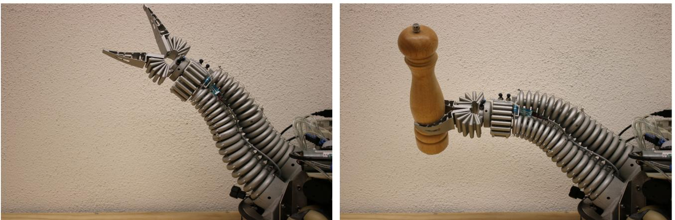
**Figure 1.1:** Compliant robot without and with load gripped. In both pictures the same control input is applied
