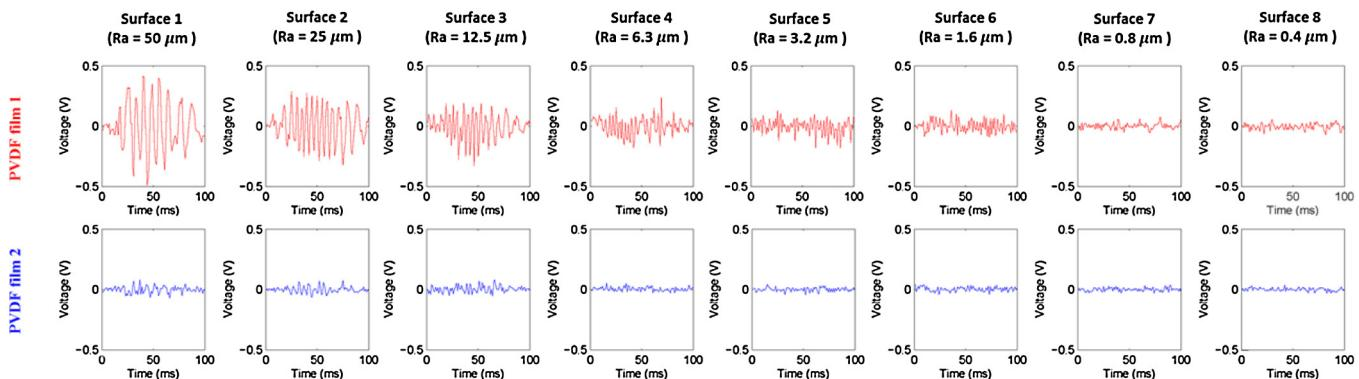
**Fig. 6.** Typical tactile signals generated by two PVDF films when laterally sliding on eight test surfaces with various roughness values.
