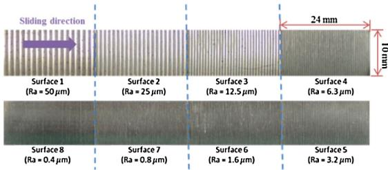
**Fig. 5.** Eight solid nickel test surfaces with roughness values  $R_a$  of 50  $\mu\text{m}$ , 25  $\mu\text{m}$ , 12.5  $\mu\text{m}$ , 6.3  $\mu\text{m}$ , 3.2  $\mu\text{m}$ , 1.6  $\mu\text{m}$ , 0.8  $\mu\text{m}$ , and 0.4  $\mu\text{m}$  were explored. The lateral sliding direction of the artificial fingertip along the test surface during the conducted experiments is indicated by an arrow.
