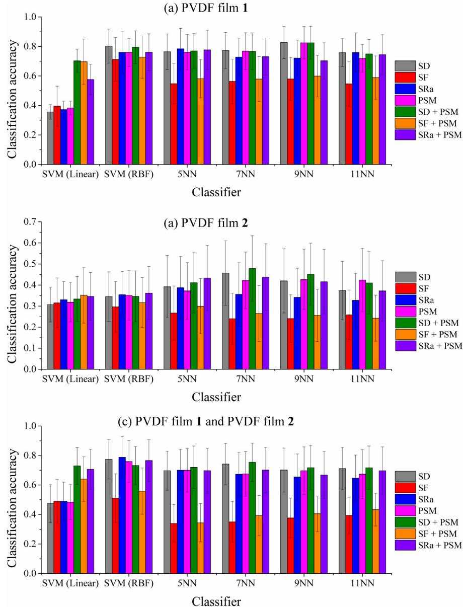
**Fig. 7.** Classification accuracy of each feature and classification algorithm with (a) only PVDF film 1, (b) only PVDF film 2, and (c) both PVDF film 1 and PVDF film 2. Error bars represent the standard error.
