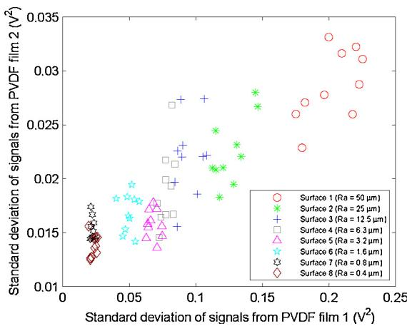
**Fig. 4.** Standard deviation features extracted from tactile signals of two PVDF films when laterally sliding on eight test surfaces with various roughness values.
