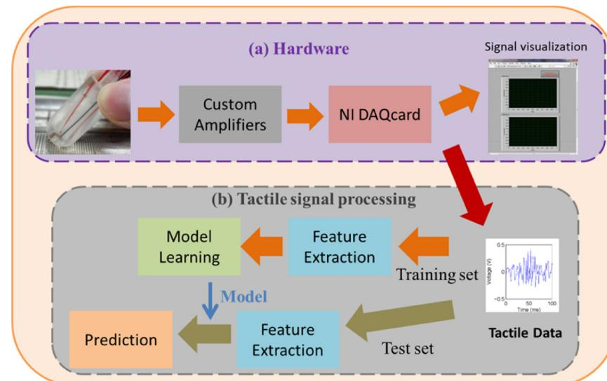
**Fig. 1.** Surface roughness discrimination approach with a bioinspired artificial fingertip. The approach consists of (a) hardware to acquire the tactile data and (b) tactile signal processing for surface roughness discrimination.
