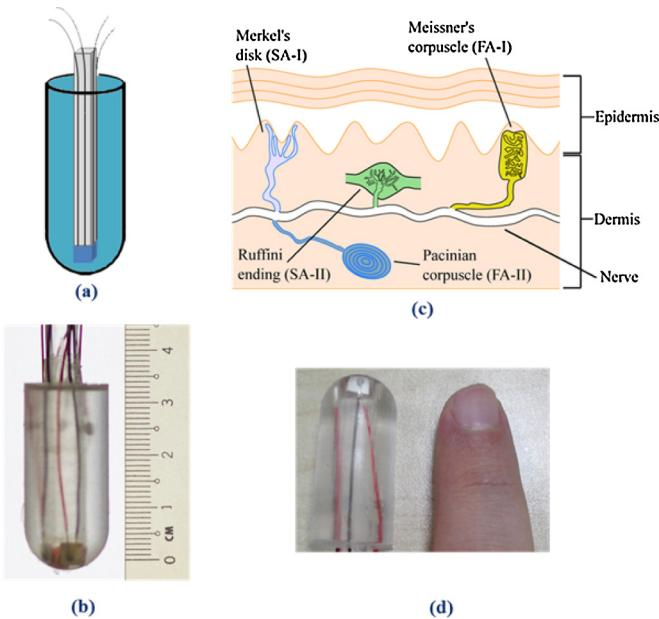
**Fig. 2.** Structures of (a) the designed artificial fingertip, (b) a developed artificial fingertip, (c) structure of human fingertip, and (d) artificial vs. human fingertip. The structures of both human and artificial fingertips contain two layers with different hardness, and a bone.
