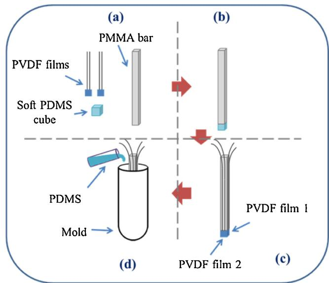
**Fig. 3.** The protocol of fabricating an artificial fingertip. (a) Components for fabricating an artificial fingertip. (b) A soft cured PDMS was bonded to the tip of a PMMA bar. (c) Two PVDF film sensors were arranged perpendicularly on the top of the PDMS cube. (d) The bar was inserted a mold of size resembles human fingertips; then PDMS mixed at a 10:1 mixing ratio was cast into it.
