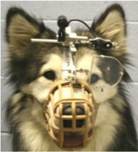
Figure 3. The eye-tracking equipment for dogs developed by Williams et al. (2011).
