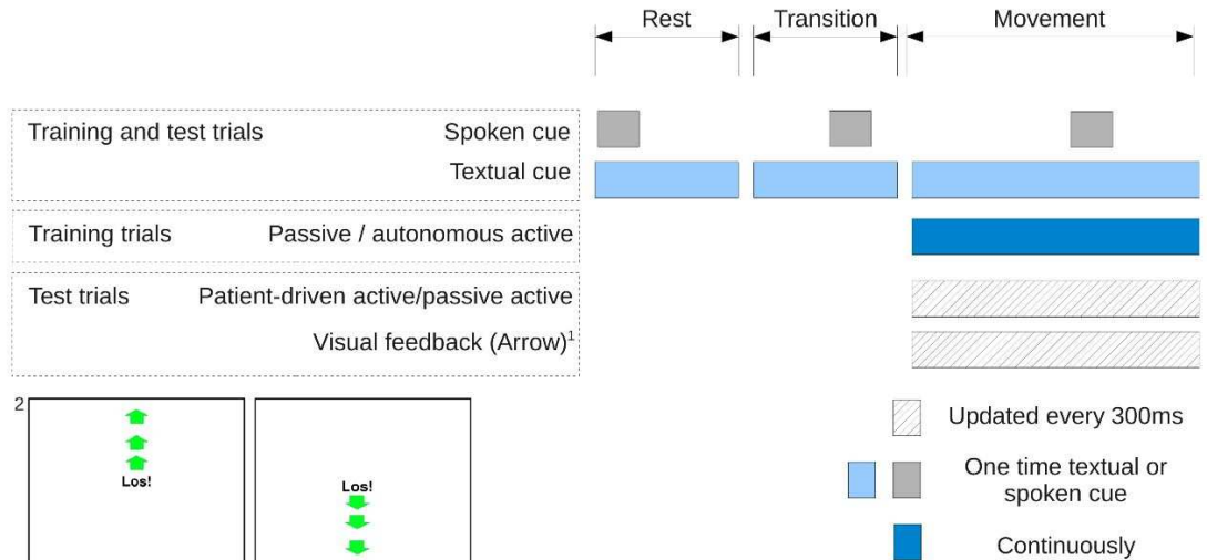
Fig. 3. Timeline of events in a single trial. Please note that the spoken and textual cues are one-time events. For movement periods of training sections, the movement of the robot is continuous, while for movement periods of test sections, the haptic and visual feedback are events that are updated every 300ms (adapted from [20]).
