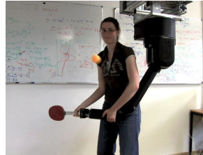
(a) Kinesthetic teach-in of the hitting skill for imitation learning.
