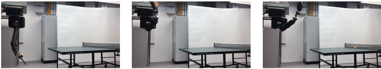
Fig. 5: A successful rollout during real robot experiments. The ball is initially on top of the egg-holder and during the movement, as a result of the acceleration of the arm, it takes-off from the robot, to be later hit by the racket towards the table. The arm then decelerates towards a safe resting posture.
