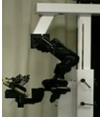
Fig. 1: Anthropomorphic SARCOS robot arm.
