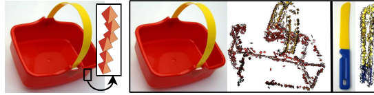
Fig. 7 ECV descriptors. Left: ECV descriptors are oriented appearance patches extracted along contours. Right: object-segmented and refined ECV descriptors via structure from motion.
