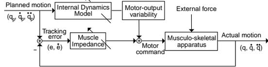
Figure 2: Control scheme of the neuro-mechanical control of human movements corresponding to Eq 5. Both the IDM and endpoint impedance are adapted to the task dynamics and the environment.
