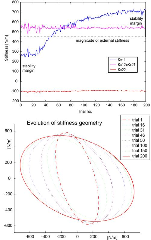
Figure 7: Evolution of stiffness during learning the DF. **A:** The  $K_x(1,1)$  parameter starts to increase around the 25th trial and converges before 200 trials.  $K_x(1,2)$  and  $K_x(2,2)$  remain constant. **B:** The effect of this evolution on the stiffness is seen by an elongation of the ellipse in the direction of the destabilizing force from the environment.
