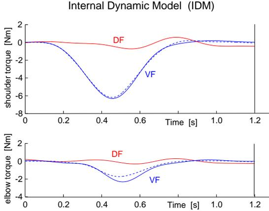
Figure 6: Internal Dynamic Model (IDM) learned during learning. Relative to the feedforward torque in the VF, the one in DF is of a small magnitude. The IDM learned in the VF (solid line) corresponds closely to the task dynamics in the VF (dashed line).
