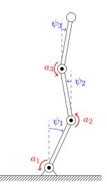
Figure 16: Balancing setup of a 3-link actuated pendulum. Each joint *i* is actuated by the signal  $a_i$ . The state of each joint is denoted by its angle  $\psi_i$  against the vertical direction. The pole is supposed to be balanced upright, that is, all  $\psi_i$  should be as close to 0 as possible.
