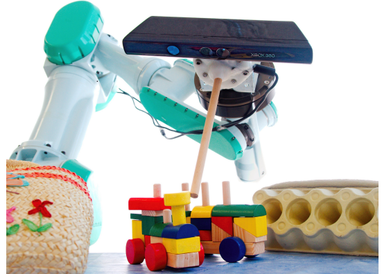
Figure 1: We use a Mitsubishi PA-10 robot arm equipped with a force-torque sensor and an RGBD camera. The robot autonomously interacts with its environment to segment a scene into objects.
