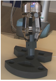
(a) Initial touching between peg and base plate.
