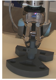
(c) Inserting peg using force feedback.
