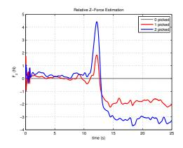
Fig. 1. z-Force along trajectory. Approximating grasp position (time 0s-10s), grasping (time 10s-12s), returning to initial position (time 12s-22s).
