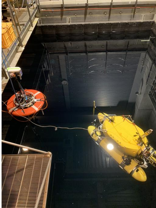
Fig. 13. Experimental facilities in the water tank. The AUV Tri-TON 2 and the autonomous surface vehicle BUTTORI are deployed in the water tank.
