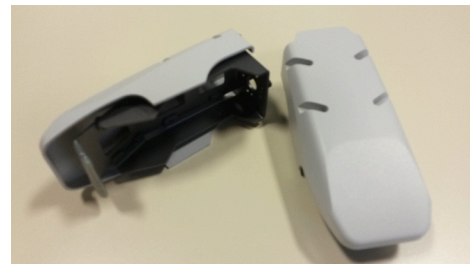
Figure 4.5: ROBOTIS-OP2 's original set of hands. This set of hands is replaced by a new one.
