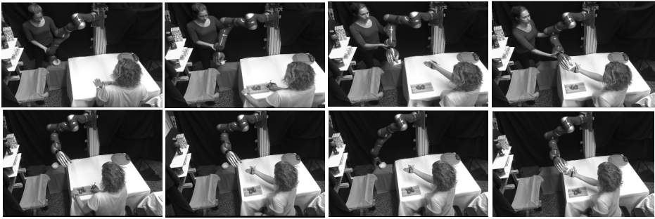
Fig. 6. (upper row) Demonstrations are recorded as human and robot trajectories. For the robot we use kinesthetic teaching and the human wrist trajectory is tracked with a motion capturing markers. (lower row) The robot performs motions according to recognized previous demonstrations.
