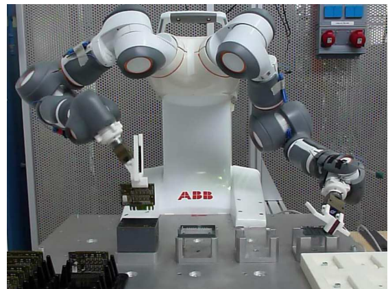
Fig. 1. ABB YuMi ( www.abb.com/yumi ), a dual-arm 7DOF manipulator, assembling a PLC I/O module employing the proposed RAS framework. The full assembly of the I/O module has been realized using the proposed approach. Two elementary operations, namely snap-fit assembly steps, are detailed in the paper to explain the proposed approach.
