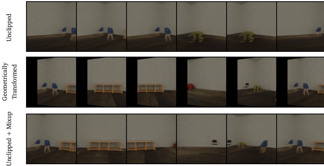
Figure 4.3.: Output Images produced by decoding pose predictions from geometrically transformed images, using unclipped variants of the encoder model. The original unclipped variant of the model is unable to make correct predictions, if fed with geometrically transformed images. The mixup variant on the other hand, is able to isolate a pose in the general vicinity of the true link pose, however, it is still off by a significant margin.
