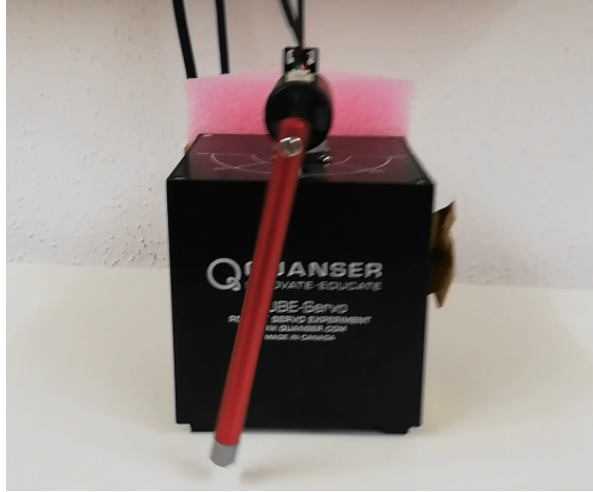
Figure 5.2: Real world Furuta pendulum used in the experiments.
