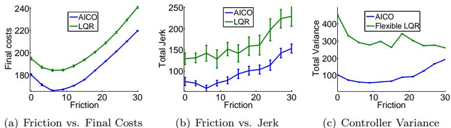
Figure 6: This figure shows the results for optimizing the link lengths and the friction coefficient of the 4-link model. Like before we used the final costs (a), the total jerk (b) and the variance of the time-varying feedback controller (c) as complexity measure.
