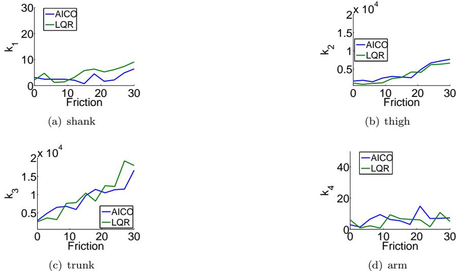
Figure 10: This figure shows the optimal spring constants for different friction coefficients using AICO and LQR.
