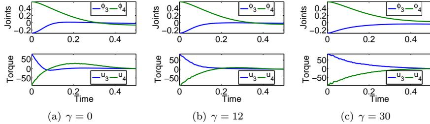
Figure 4: The plots show the mean trajectories of the hip ( $\phi_3$ ) and the arm ( $\phi_4$ ) joints over 100 runs for the first 0.5s, where we used the AICO approach for the friction coefficients  $\gamma = 0$ ,  $\gamma = 12$  and  $\gamma = 30$ .
