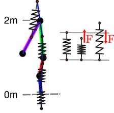
Figure 8: This figure illustrates the 4-link robot model endowed with linear springs which are mounted at the midpoints of the joints. These springs support the control of the 4-link robot as they push the robot back into its upright position. Due to the calculation of the spring length displacements, the springs act non-linearly on the joint torques.
