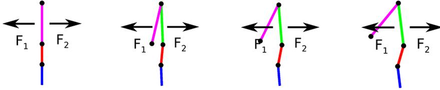
Figure 2: This figure illustrates different initial postures of a 4-link pendulum modelling a humanoid robot (70kg, 2m). The robot gets pushed with specific forces, i.e.  $F_1$  and  $F_2$  and has to move such that it maintains balance. At the end of the movement the robot should stabilize at the upright position.
