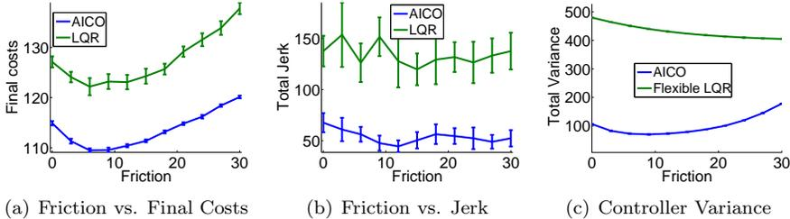
Figure 9: This figure shows the results for optimizing the spring constants and the friction coefficient of the 4-link model. We used the final costs (a), the total jerk (b) and the variance of the time-varying feedback controller (c) as complexity measure.
