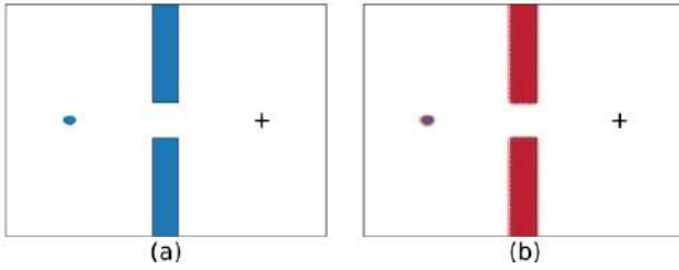
Figure 4. 2D navigation task. (a) Environment. The robot is represented by a blue circle, the walls by the rectangles and the target by the cross. (b) spherical obstacle bodies for the robot and the walls.
