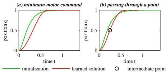
Fig. 1: (Color online) This figure shows the initial and the final trajectories for the two motor control tasks. Both start at 0 and have to go to 1 with minimal accelerations. From  $T/2 = 0.75$  on the trajectory has to be as close to 1 as possible. For the passing through task the trajectory additionally has to pass through  $p_M = 0.5$  at time  $M = 7/40T$  indicated by the circle.
