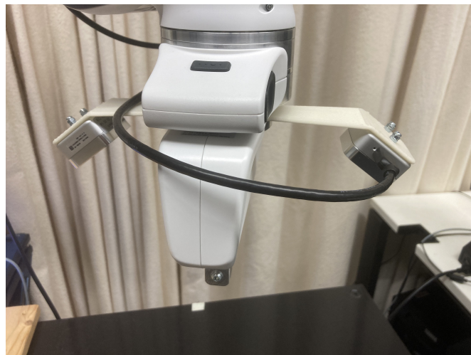
Figure 4.2: The D405 cameras mounted above the EE, looking between the fingers. The mount is 3D printed. The angle is set at 55^\circ , so that only the block and the fingers of the gripper are in view.
