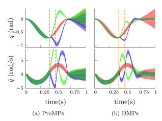
**Fig. 8** Robustness evaluation. We applied a perturbation between the dashed lines with an amplitude of  $P=200(m/s^2)$  (green), or an amplitude of  $P=-200(m/s^2)$  (blue). The ProMPs (a) show compliant behavior but pass through the via-point accurately. The DMPs (b) are much stiffer and compensate the perturbation faster, before the via-point was reached. The DMPs exhibit a less efficient recovery strategy due to the higher actions.
