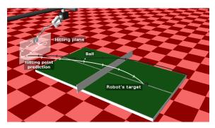
Fig. 13 The simulated table tennis setup. (left) Shown are the robot arm mounted on linear axis, the ball position, the hitting plane in which the robot will try to hit the ball, and the hitting point prediction. Due to the induced noise in our simulation the desired and actual hitting points may differ. On the opponent's side, we can see the robot's target for this simulation. In our experiments, we use 15 different combinations of initial ball positions and targets covering most of the table.
