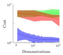
Fig. 10 Evaluation of the reproduction cost versus the number of demonstrations provided for training on the 7-link task-space via-point task. We present the results using ProMPs (blue), the Inv. Cov. Ctl. (red) [5], and DMPs (green) [17]. The cost is averaged over 200 reproductions for every approach and over 10 trials.
