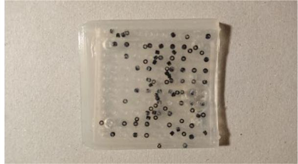
(b) An illustration of the issue in which the micro breads were continuously losing their initial positions inside the silicon layer.
