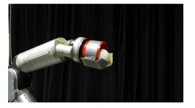
• An end effector with cup and a simple holder attached to it
