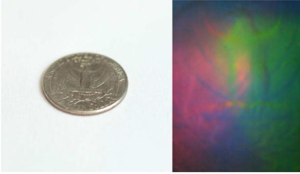
Fig. 2. Output of the real DIGIT sensor (image taken from [8]). Touching the coin with the sensor causes the gel to deform according to the coin’s surface geometry. Fine details of the coin are clearly visible in the reflections of the LEDs’ light from the gel.
