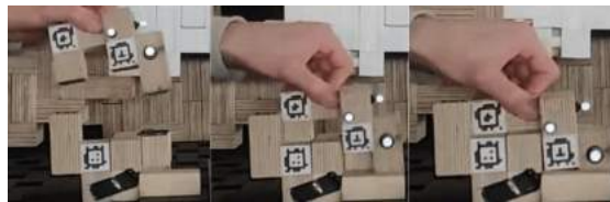
Figure 3.4.: A human performing the task repeatedly while the trajectory of the block is recorded by the tracking system. The state space is sampled close to the goal state.
