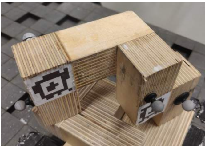
(a) Close up view of the SL-Blocks that is joined in our simplified setup. The QR-codes on the block are AprilTag fiducial markers. The grey balls are OptiTrack markers. Because the AprilTag marker tracking is not very precise and robust to changes in lighting and occlusions OptiTrack was used. But as the tracking balls make the assembly of multiple parts impossible AprilTags or even markerless object-based tracking stays relevant.
