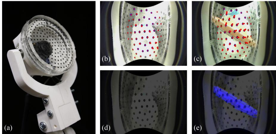
**Fig. 17.** The camera image from the Finger Vision sensor (a). Blob detection with no object (b), applied force to an object, red lines indicate the measurements in the direction (c), no object in slip-detection mode (d) and an inserted object recognized by the sensor, blue pixels shows the object (e).
