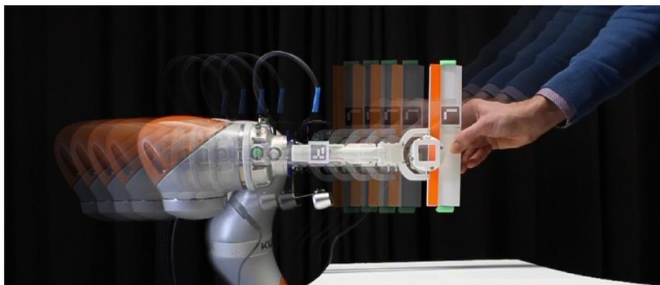
**Fig. 16.** Human applying force by pulling the object and robot following in the desired direction.
