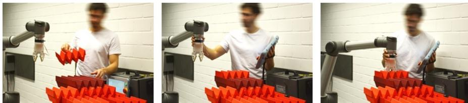
**Fig. 13.** Digitization of new module position in compliance mode: human places a new module (1), human moves robot to location of module (2), new position is saved (3).
