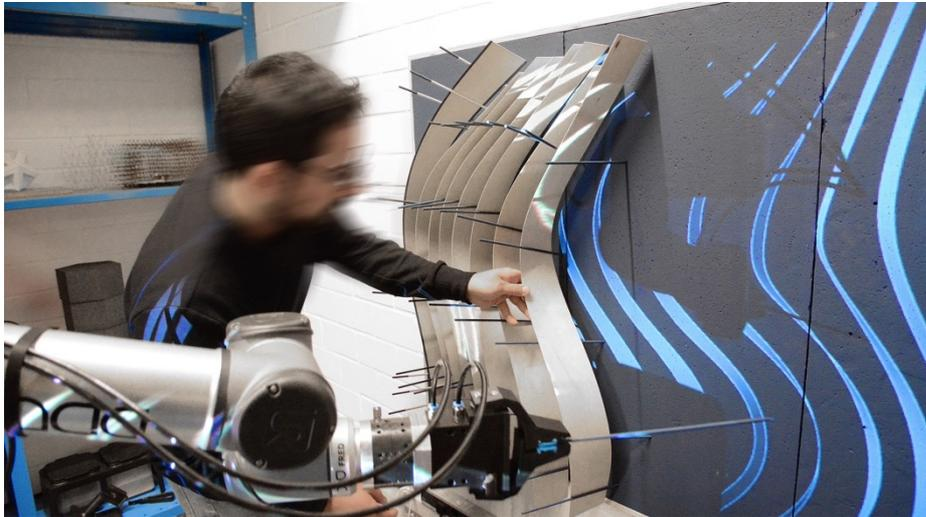
**Fig. 5.** Division of task in a collaboration assembly, composed of rods and lamellas and augmented by a projection.
