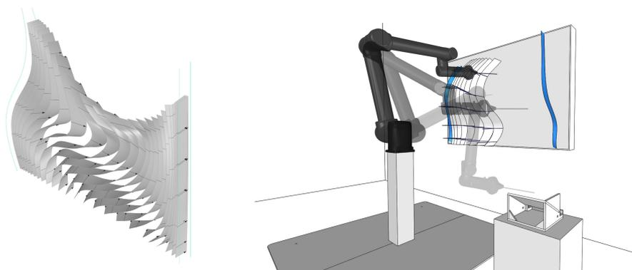
**Fig. 8.** Robot path generated based on the interpolated lamellas (1) and simulation of the robot program (2).
