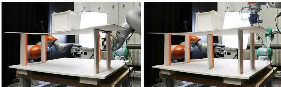
**Fig. 19.** The deformed slab without any support (1) and a wall component inserted below the point with the highest load (2).
