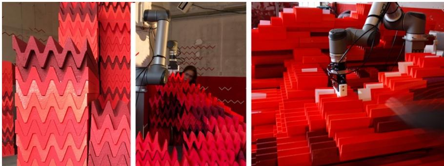
**Fig. 10.** Modules in compact arrangement (1), robot in compliance mode to capture module position (2), top layer of modules marked for robotic repositioning (3)
