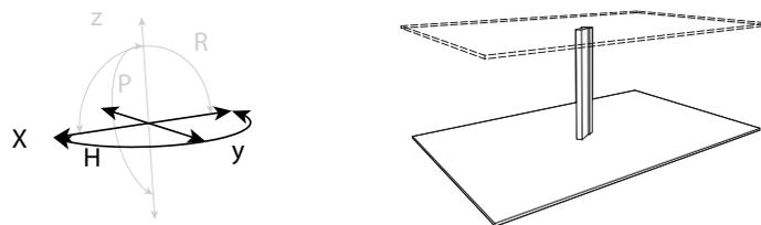
**Fig. 18.** Three degrees of freedom of wall element being placed between two slabs.
