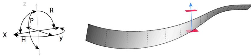
**Fig. 6.** Degrees of freedom of rods that are to be positioned by the robot following the geometrical principle of a ruled surface.
