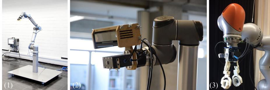
**Fig. 4.** Robots with different sensor types: position sensor for self-aware location picking (1), Microsoft Kinect V2 depth camera (2), FingerVision gripper for force and slippage detection (3)
