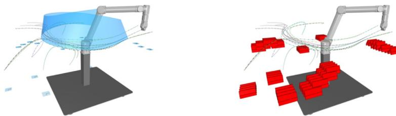
**Fig. 14.** Depicted planes from the assembly and surface constraining the robot path (1), digital representation of taught module positions (2).
