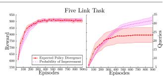
Fig. 10: Performance of EPD ( $\kappa = 0.02$ ) and PI ( $\lambda = 1.1$ ) on the five link task. EPD and PI show similar reward while EPD requires less total user inputs. Since PI does not have a notion of a policy, it keeps optimizing the reward model after the policy has converged.
