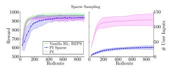
Fig. 6: Results of comparing our acquisition algorithm to the standard acquisition algorithm. Our algorithm collects sparse user queries and does not ask for any user queries after a PS iteration if the outcome that maximizes the AF has already been queried before.
