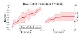
Fig. 15: Performance of Expected Policy Divergence on the real robot pendulum swing-up task. EPD learns to successfully swing up the pendulum on the real robot with an average of about eight user queries. Results averaged over three trials.
