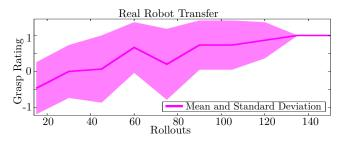
Fig. 17: Performance of one trial on the real robot system. The robot uses the reward function learned in trial one of the original task to learn to grasp a new, unknown object (a wooden pestle as shown in Fig. 3). For this trial, we did not allow any expert queries. The robot successfully learned to grasp the object.
