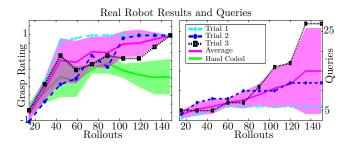
Fig. 16: The real robot successfully learned good grasps in all of the three trials. The grasp rating scheme is described in Fig. 3. In the last trial, one joint failed, represented by a spike in expert queries. The robot successfully adapted the reward function to recover from the hardware failure. We also show the average performance of a naive hand coded reward function.
