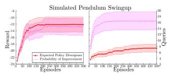
Fig. 14: Performance of EPD ( $\kappa = 0.001$ ) and PI ( $\lambda = 1.1$ ) on the simulated pendulum swing-up task. EPD achieves slightly better performance while requiring less than half the number of user queries.
