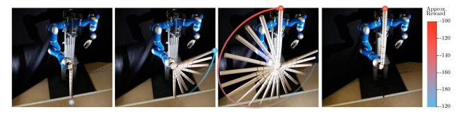
Fig. 13: Picture of the robot performing the swing-up task. The initially suspended pendulum is first counter-clockwise to build momentum and then swung clockwise to the upright position. The heat map gives an indication of the approximate trajectory reward if the swing-up would reach up to the indicated position.
