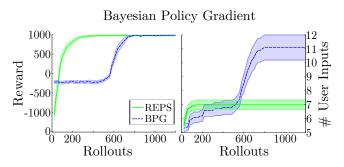
Fig. 9: Performance of REPS and BPG on a via point task.
