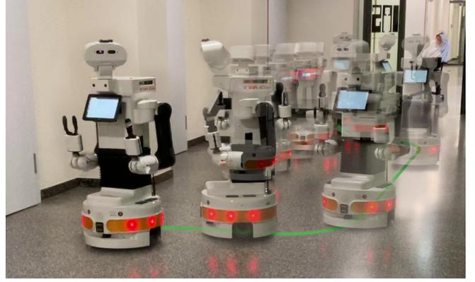
Fig. 9. TIAGo robot performing an overtake by planning under uncertainty and collision probability bounds
