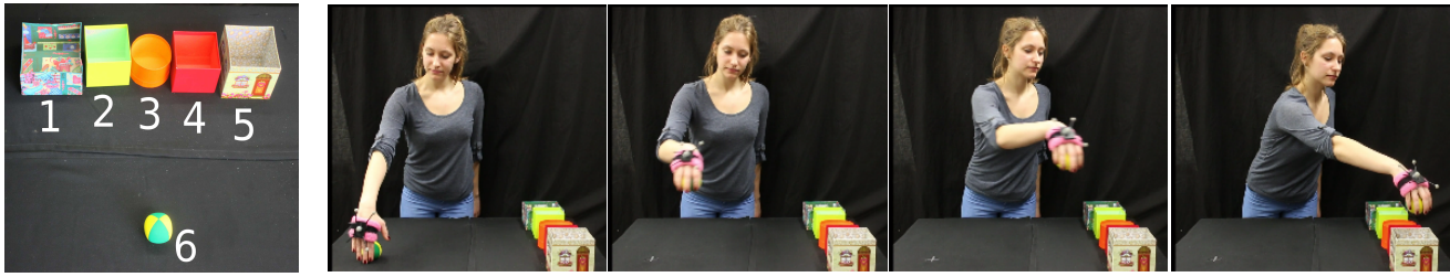
Fig. 5. We consider a pick-and-place scenario with a ball and five boxes as illustrated on the left. Human demonstrations, as shown on the right, are recorded using an OptiTrack motion capturing system for the wrist position. The proposed algorithm is evaluated on a 7DoF Kuka Lightweight arm to achieve robot motions that are similar to the demonstrated motions, while generalizing to different work space settings, such as obstacles, not present during the original demonstrations, and deliveries to different boxes.
