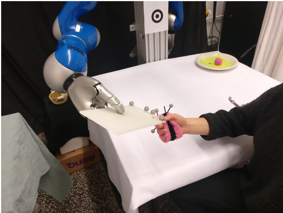
Figure 3.4: This photo was taken while a subject is performing the “board” gesture for recording the salad data set. The grey markers were used to track the position of the hand, and the robot was moved manually as it would in the real scenario in order to observe realistic behavior of the subjects.
