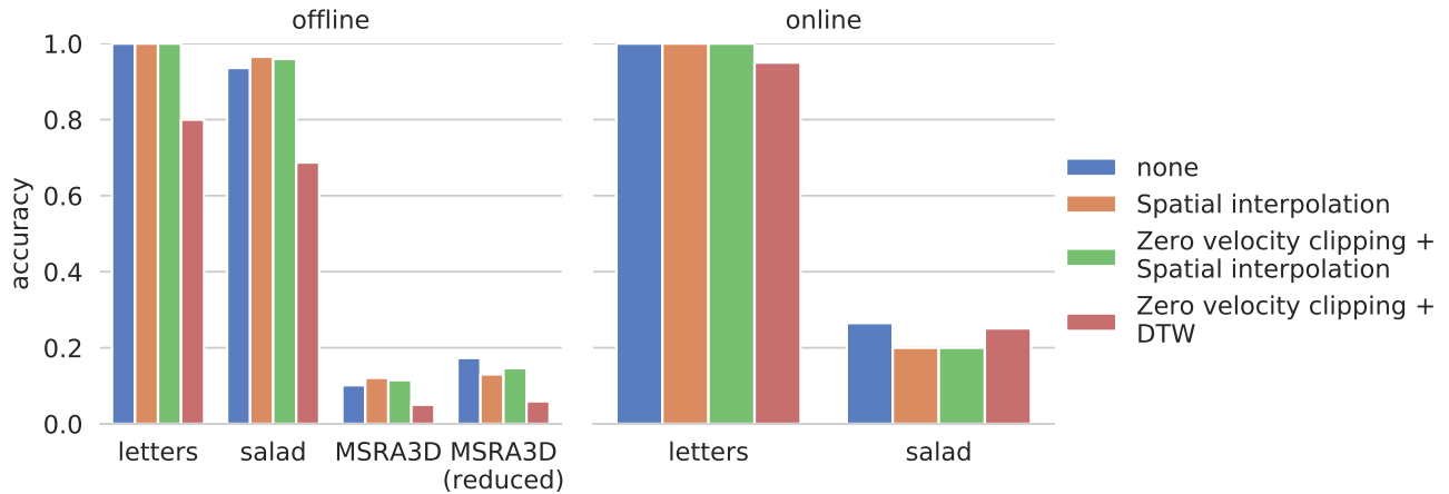
Figure 4.14: Classification results on all four data sets using SVMs in the trajectory space, i.e. without a prior weight space transformation. The evaluation is given for each of the previously selected time sequence alignment methods. The trajectory was sampled at 80 points in time. As before, online evaluation was not performed on the MSR Action3D data set.
