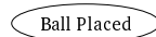
Figure 4.1.: The initial BT created by the PA-BT algorithm consisting only of the goal condition.
