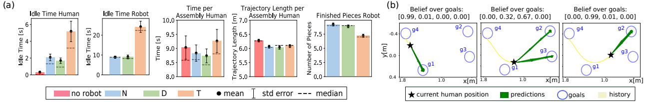
Fig. 6. (a) During the user study, we recorded and evaluated motion data from the subjects and the robot for the different adaptation modes, namely no reaction (N), spatial deformation (D) and temporal scaling (T). (b) Using a probabilistic goal directed motion model, that was learned from observation, the belief over the goals and the predictions (green) change given an observed human trajectory (yellow) and the current position (black star).
