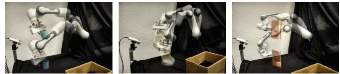
Fig. 3: The figures show overlays of the successful grasp execution sampled with GDN for different real-world objects.
