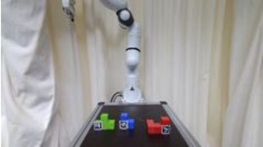
Figure 6.2.: The experimental setup used for the recording of real videos. The Ubongo3D shapes are used, and an ArUco marker is placed on each of them to recover the ground truth pose.
