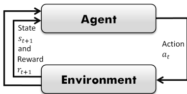
Figure 1. The Agent-Environment Interaction Cycle. The agent executes action a_t at time step t . The environment returns the new state s_{t+1} with reward r_{t+1} which are based on the executed action. Graphic based on (Sutton & Barto, 2018).
