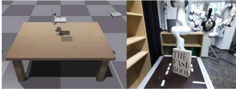
Figure 5.1.: Grasp testing in the Isaac Gym simulation environment (left) and the real world (right).
