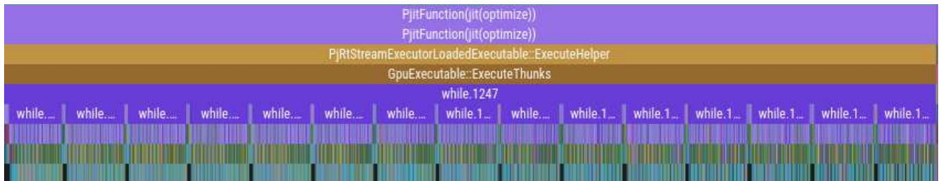
Figure 6.6.: GPU trace of a single jit-ed optimization step as in Algorithm 5 running base MPPI over 15 horizon steps on the FR3 Push T task. The 15 steps encapsulating sim_steps_per_control_step physics steps (small purple chunks) dominate the runtime.
