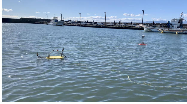
Figure 10: We deployed Tri-TON and BUTTORI for alignment control experiments in Hiratsuka, Japan. The yellow platform on the left side of the figure is Tri-TON, and the red platform on the right side is BUTTORI.
