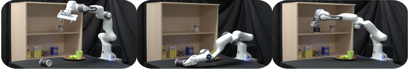
Fig. 1: Pick and place task in which the robot has to pick a mug and move it to the target pose (in the shelves) without colliding. We exploit diffusion models for jointly optimizing both grasp and motion and show the successful trajectory from left to right.
