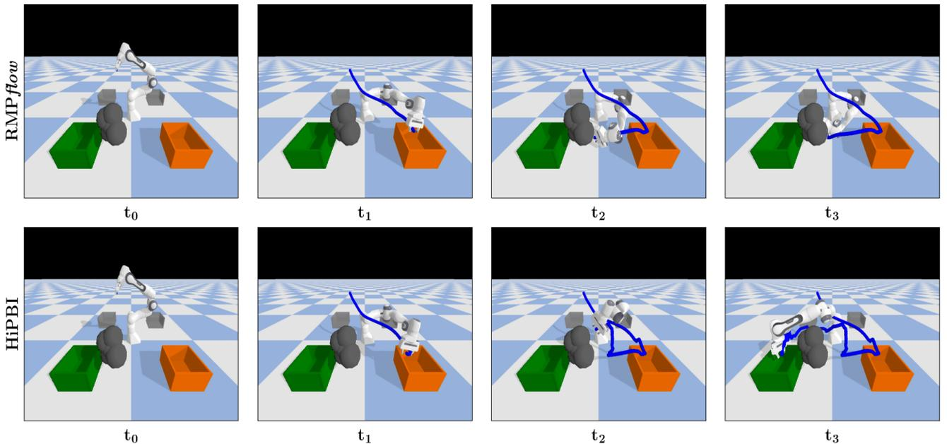
**Fig. 4:** Manipulation environment in which the intermediate (orange) and target (green) boxes are randomly selected out of four boxes. Five randomly generated grey obstacles obstruct the path of the 7DoF manipulator robot. With blue, we denote the executed trajectory. **Top.** Performance of Riemannian motion policies (RMPflow) method that gets stuck in a local optimum. **Bottom.** Performance of our proposed HiPBI, that successfully discovers an obstacle-free path to the target.
