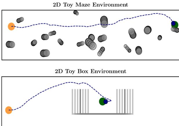
**Fig. 2:** 2D Toy environments for planar point-mass navigation. The orange dot denotes the start and the green one the goal location. **Top.** The toy maze environment with dynamic obstacles. **Bottom.** the toy box environment, in which a box moves horizontally at a constant speed. The goal is fixed in the center of the moving box.
