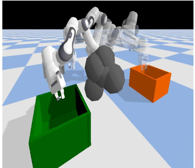
**Fig. 1:** A sequence of the reactive motion of a 7DoF manipulator robot. The robot starts moving from the orange box toward the green box. Our proposed method enables a reactive motion that avoids collisions with the grey obstacle and overcomes local minima resulting from multiple constraints.
