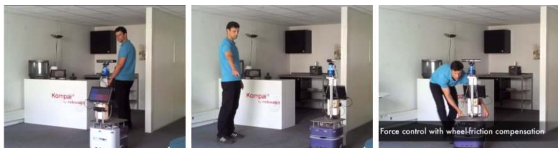
Figure 2.2.: Interaction modalities: person following (left); pointing control (center); direct physical interaction (right) [3]
