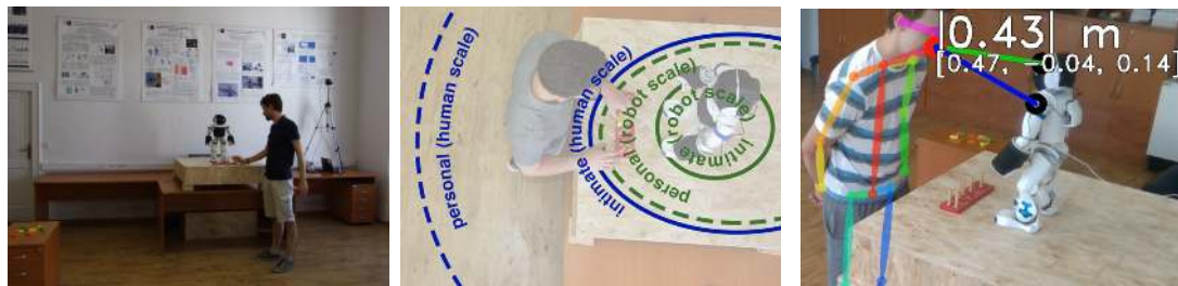
(a) Experiment setup (b) Spatial zones of human and robot (c) Participant gazes at robot
