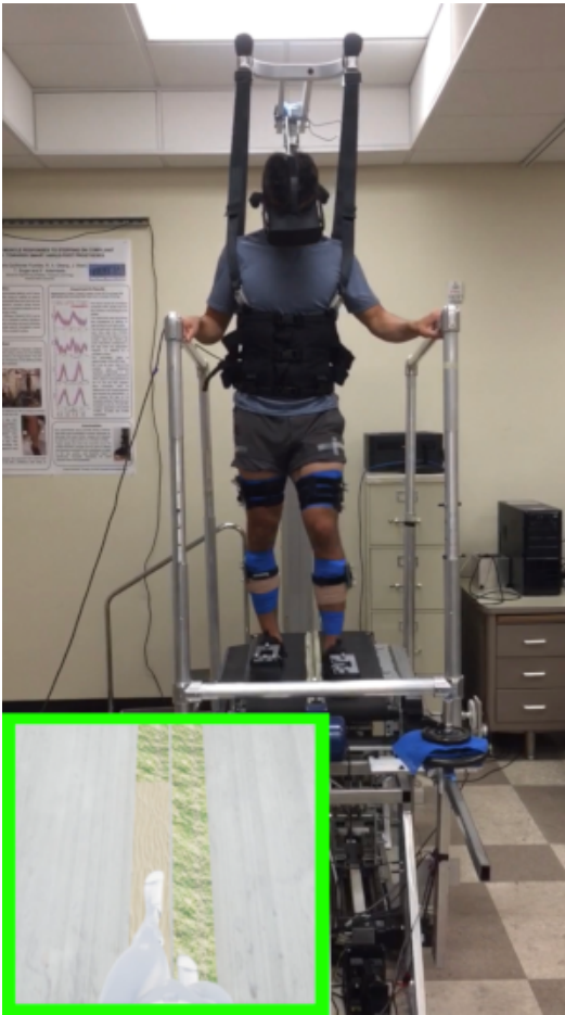
Fig. 1. Subject Walking on the Variable Stiffness Treadmill (VST) while wearing the virtual reality headset (Oculus Rift).
