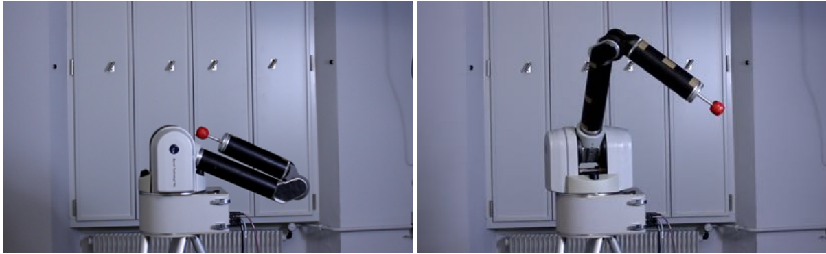
Figure 2.3.: Left: The physical Barrett WAM 4DoF robot in the lab of IAS in its resting position. Right: The WAM during execution of a trajectory. The base joint is rotated, the arm is tilted and rotated, the elbow joint is unfolded.
